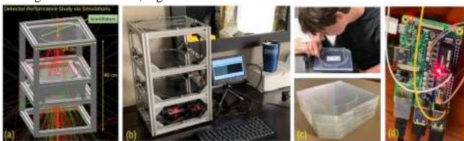
Figure 3. Low-cost and portable cosmic ray detector. (a) Simulation study of the detector efficiency and acceptance; (b) Demonstration of a running detector at the International Cosmic Ray Conference, Madison, Wisconsin, July 2019; (c) Making scintillator tiles by an undergraduate; and (d) Low cost readout unit.
