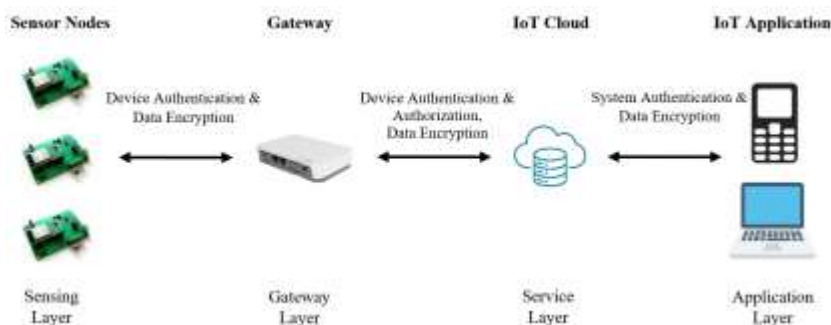
Fig. 2. EIoT architecture with a high level of security. Source: Redrawn by authors based on [9].
