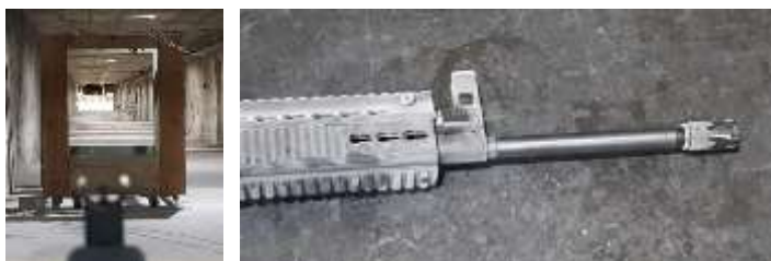
Fig.5. Shooting through the velocity barrier, set at 10m, after reaching -50 °C – left, heating of the rifle barrel and the ice melting – right
